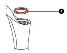
The old sealing rings and dust seals must not be used again.
