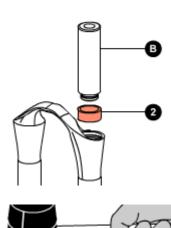
Using a hammer knock the introducer  $(\boldsymbol{B})$  into the arch-slider assembly.
