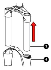
Dismantling: Dismantling the right pumping element and valve
