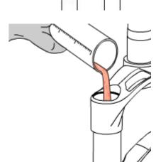
A lower or higher volume or a type of oil other than the one recommended can change the behaviour of the fork in every phase.
