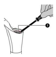
Protect the upper part of the slider with the special tool ( $\bf A$ ).
