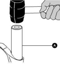
Using the short introducer (B) fit the top bush (2).
