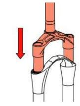
In a graduated recipient, prepare the quantity of oil to pour into the fork leg (see table). Pour roughly 1/3 of the oil required into each stanchion, then pump the fork a few times to eliminate any traces of air.
