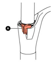
The brake cable must never touch the crown and stanchions.
