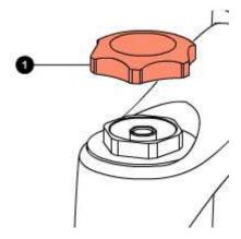
Using a small pin screwdriver, blow the air off the fork leg, pushing on the air valve. Fully unscrew lock cap (2) with a 21mm socket spanner. Remove lock cap (2).
