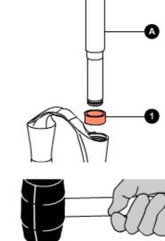
Using a hammer knock the introducer (A) into the arch-slider assembly.
