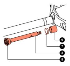
If the piston segment  $(\mathbf{8})$  is damaged, you can prize it off with a small flat-tip screwdriver.
