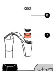
Using a hammer knock the introducer (B) into the arch-slider assembly.
