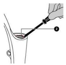
Protect the upper part of the slider with the special tool (  ${\bf A}$  ).
