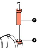
Pull the extractor rod so that the upper face of the washer stops against the lower face of the guide bush. Insert the aluminium bush (**A**) in the seat of the sealing ring.
