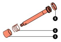
Assemble the valve unit in this order: bushing (4),valve (5), three-point ring (6), and check that the parts are oriented as shown.
