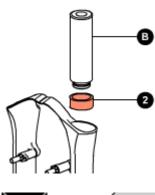
Using a hammer knock the introducer  $(\boldsymbol{B})$  into the arch-slider assembly.
