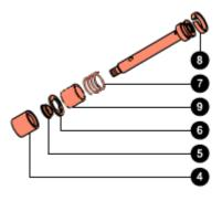
If the piston segment (8) is damaged, you can prize it off with a small flat-tip screwdriver.
