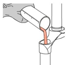
A lower or higher volume or a type of oil other than the one recommended can change the behaviour of the fork in every phase.
