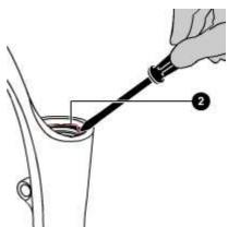
Protect the upper part of the slider with the special tool (**A**). With a screwdriver, prize off the sealing ring (**3**). Remove the sealing ring (**3**).
