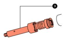
Remove bushing (4), the rebound spring (7) and the preload tube (9) (only for models with 105mm travel) from the pumping element.
