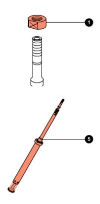
The ETA cartridge (5) has been sealed through machining and cannot be overhauled. In the case of faults or a malfunctioning, this cartridge must be replaced.
