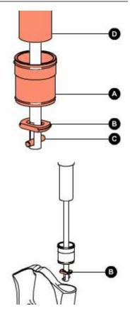
Pull the extractor rod so that the upper face of the washer stops against the lower face of the guide bush. Insert the aluminium bush ( $\bf{A}$ ) in the seat of the sealing ring.
