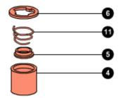
Insert the pre-assembled value in the piston rod from the three-point ring side as shown. Insert the value and the pumping element (3) into the stanchion.
