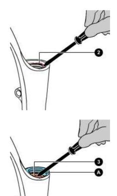
The old sealing rings and dust seals must not be used again.
