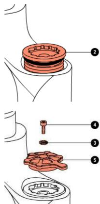
Fit the ETA control knob (5), washer (3) and screw (4). Using a 2mm Allen key, tighten the knob fixing screw (4) to the recommended tightening torque (2 Nm  $\pm$  0.5).
