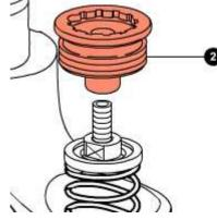
Screw the lock cap (**2**) down on the rod of the ETA cartridge without tightening being very careful not to damage the O-ring.
