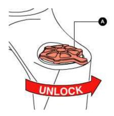
NEVER use the "LOCK" position when riding on steep downhills. Failure to comply with these instructions could cause your fork not to react safely enough when hitting an obstacle, resulting in a loss of control of the bicycle, damage and serious or lethal injury.
