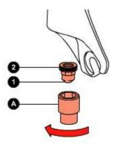
Using the special 12mm spanner (**A**), loosen the left bottom nut (**1**). Pull out the left bottom nut (**1**) complete with O-ring (**2**).
