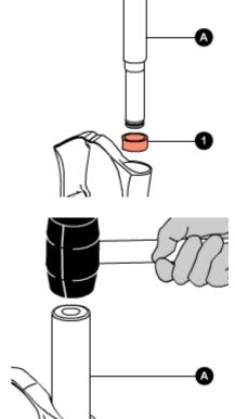
Using a hammer knock the introducer (A) into the arch-slider assembly.
