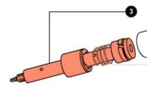
Take great care not to damage the segment and if necessary use a small flat-tip screwdriver to help the piston of the pumping element into the stanchion.
