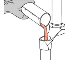
A lower or higher volume or a type of oil other than the one recommended can change the behaviour of the fork in every phase.
