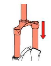
In a graduated recipient, prepare the quantity of oil to pour into the fork leg (see table). Pour roughly 1/3 of the oil required into each stanchion, then pump the fork a few times to eliminate any traces of air.
