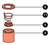
Insert the pre-assembled valve in the piston rod from the three-point ring side as shown. Insert the valve and the pumping element (3) into the stanchion.
