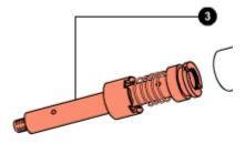
The piston of the pumping element should enter the stanchion without any interference.
