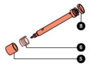
Assemble the valve unit in this order: bushing (4),valve (5), conical spring (11), three-point ring (6), and check that the parts are oriented as shown.
