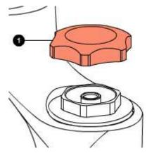
Using a small pin screwdriver, blow the air off the fork leg, pushing on the air valve. Fully unscrew lock cap (2) with a 21mm socket spanner. Remove lock cap (2).
