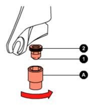
Using introducer (A) insert the dust seals (11) in their seats.
