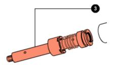
Remove bushing (4), the rebound spring (7) and the preload tube (9) (only for models with 105mm travel) from the pumping element.
